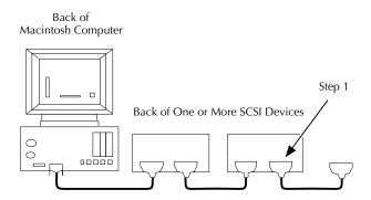
2. Attach the other end of the cable to either of the identical SCSI ports on the back of the Scanner. Seat the connector firmly and pinch the wire clamps shut.
